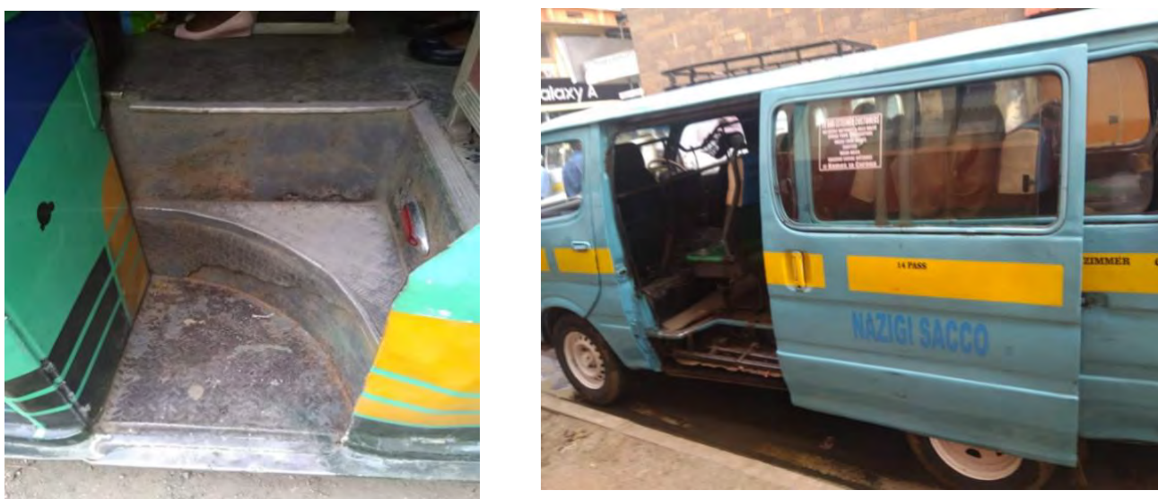
Figure 21: High staircases on Public Service Vehicles
